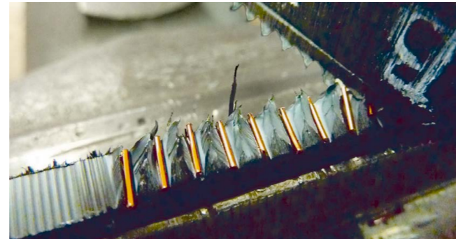
Fracture properties of SIMOFUSE® weld sample using torsion shear test.
