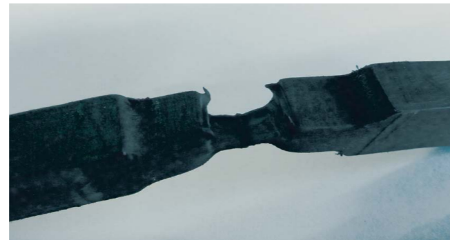
Test piece after creep fracture in weld area.
