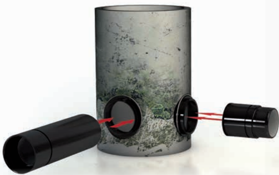
Fig. 3: Smooth pipe end is welded to the shaft connection; SIMOFUSE® End previously removed is welded to opposite shaft connection using the smooth end of the pipe
