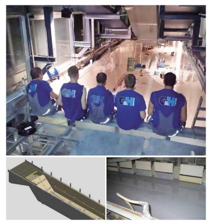
Top: cathodic electrocoating bath with SIMONA® PP AlphaPlus® inliner; bottom left: technical drawing of the cathodic electrocoating bath; bottom right: cathodic electrocoating bath filled with liquid paint
