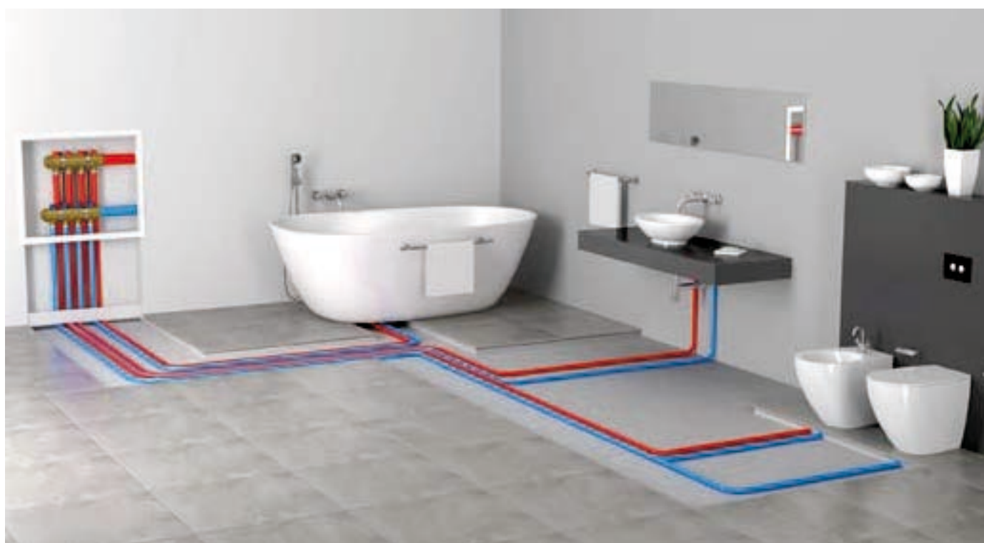
Water supply system realized with multilayer pipe insulated or with coloured protective conduit
