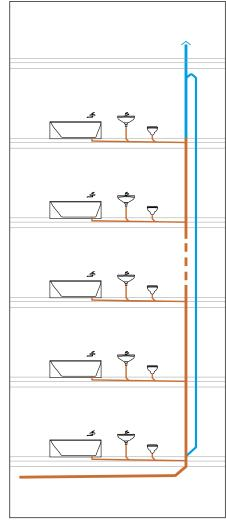
Drainage capacity **40% greater** than systems with primary ventilation.
