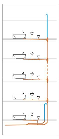
Drainage capacity **120% greater** than systems with primary ventilation.
