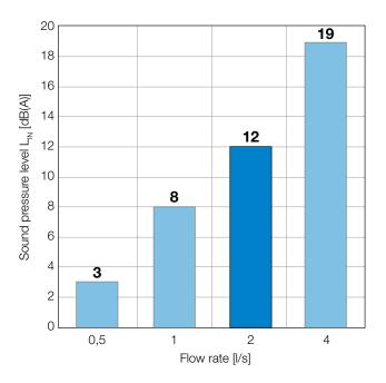
Sound pressure levels expressed in dB(A) measured on the ground floor behind the installation wall for pipe diameter 110 mm in compliance with DIN 4109 and EN 14366. These results were obtained by the Fraunhofer Institute of Stuttgart using two soundproofing pipe clips on each floor.
